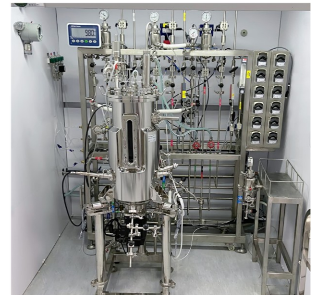
30L Bottom magnetic mixing bioreactor
