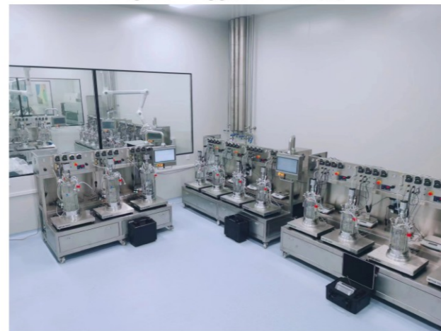
BLBIO-XGJ-11-plus Elevenfold mechanical mixing glass fermenter (5L)
