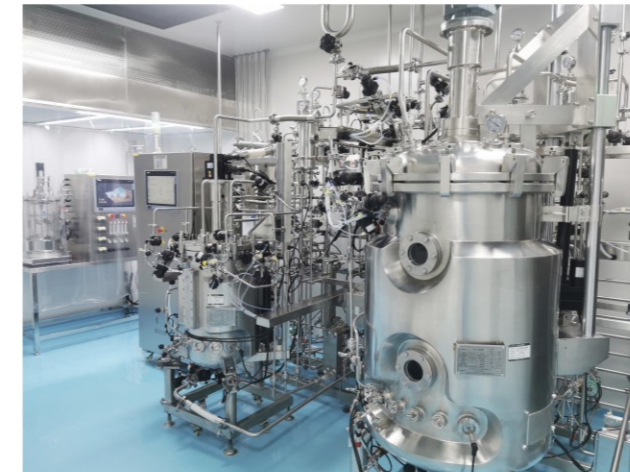
50L-250L Secondary Mammalian Cell Bioreactor
