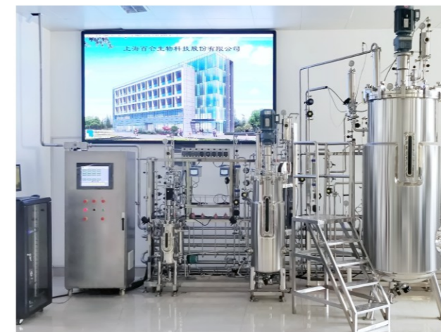
BLBIO-10SJDU-100SJDU-500SJDU 10L-100L-500L Three stage fermentation system
