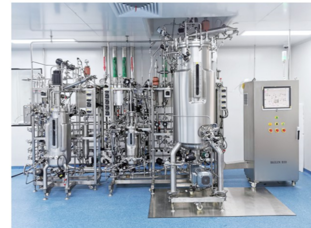
BLBIO-200SJBA 200L Bottom mechanical mixing stainless steel fermentation system
