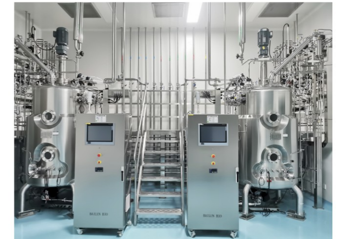
1000L Secondary Mammalian Cell Bioreactor
