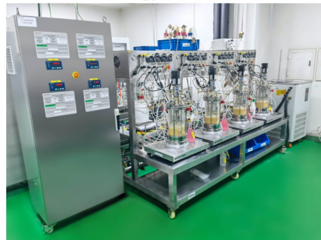
BLBIO-XGJ-4-plus Quadruple mechanical mixing glass fermenter (5L)
