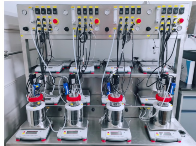
BLBIO-XGC-4-plus Quadruple mechanical mixing glass fermenter (500ML)
