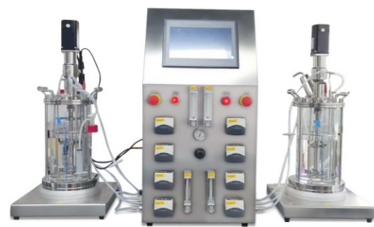
BLBIO-XGJ-2-A Double mechanical mixing glass fermenter (desktop)
