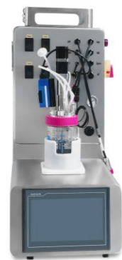
BLBIO-0.2GJ-mini 0.2L mechanical mixing glass bioreactor
