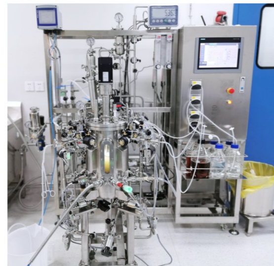
BLBIO-30SJA-FMT 30L Metabolic flow automatic bioreactor system
