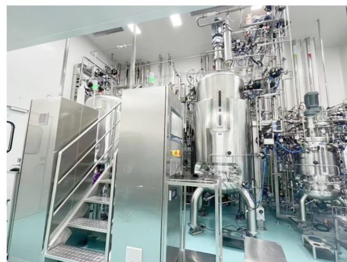
70L-1500L Top magnetic mixing bioreactor
