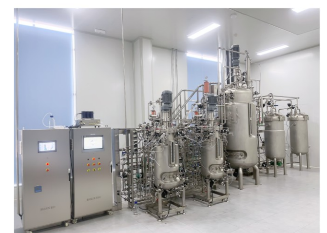
BLBIO-100SJA-100SJA-1000SJA 100L-100L-1000L Double secondary fermentation system
