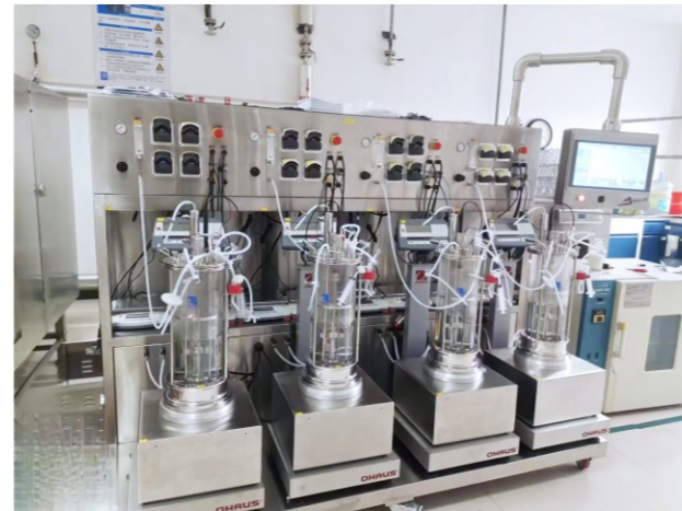
BLBIO-XGC-4-plus Quadruple magnetic mixing glass fermenter (5L)
