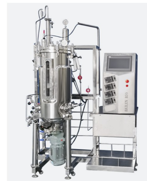
BLBIO-50SC 50L Bottom magnetic mixing fermentation system
