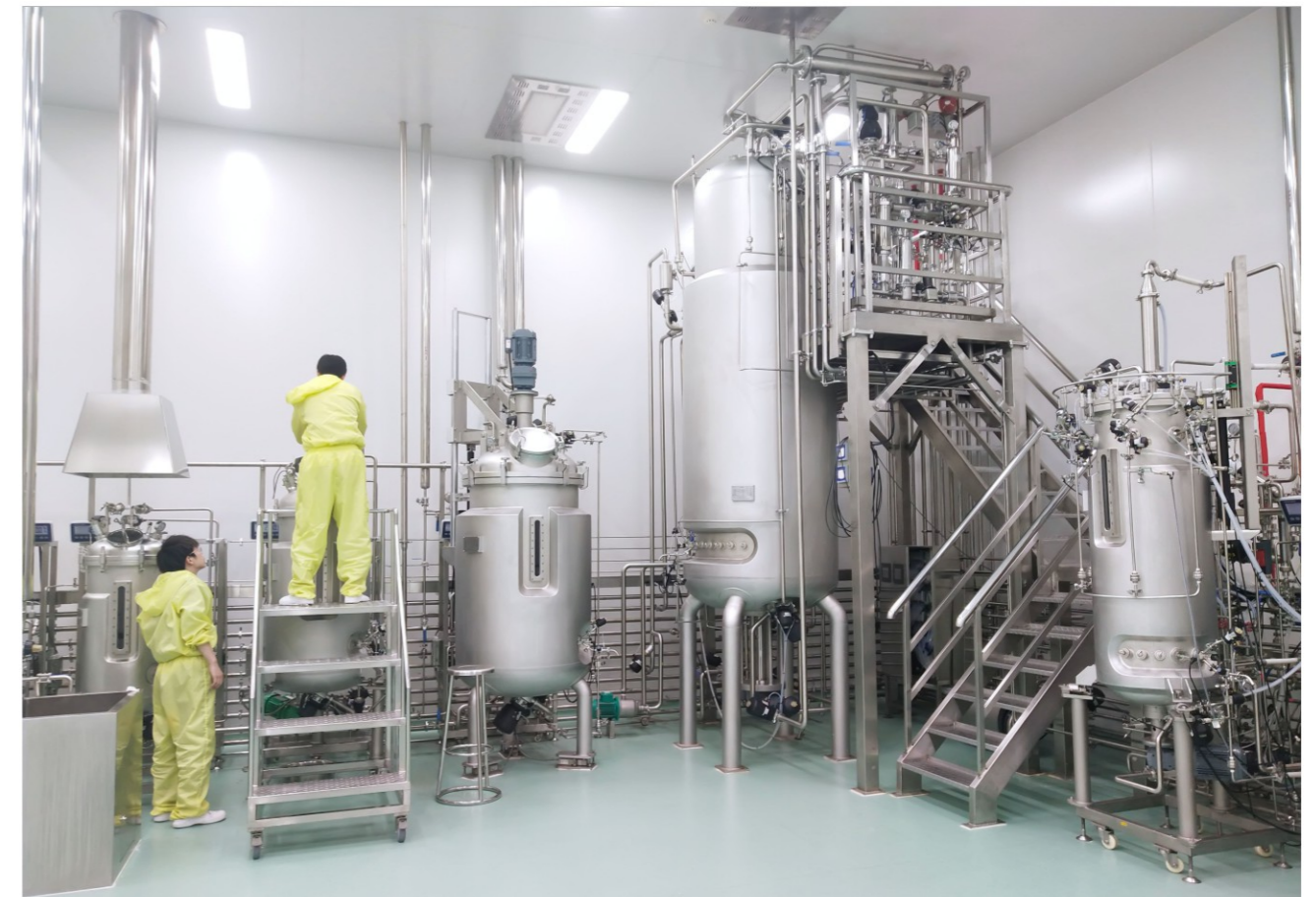
BLBIO-300SJBA-3000SJBA 300L-3000L Bottom mechanical mixing stainless steel fermentation system
