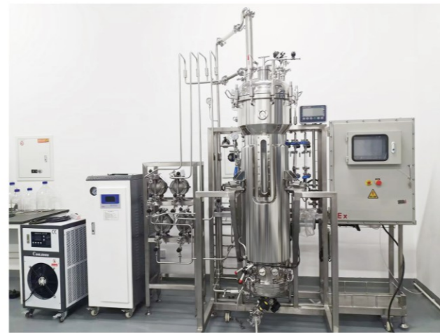
BLBIO-100SQA 100L Air lift mixing stainless steel fermentation system
