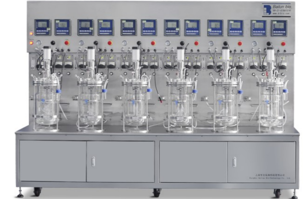
BLBIO-XGJGG-6 Sextuple double wall glass fermenter (5L)
