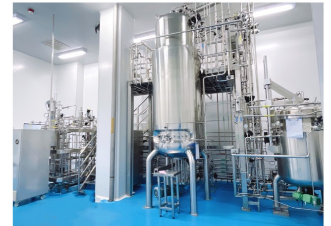
BLBIO-2000SJBA 2000L Bottom mechanical mixing stainless steel fermentation system
